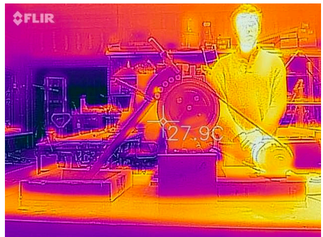
Figures A11-A12: Infrared camera renderings and heat maps following braking procedure trials
